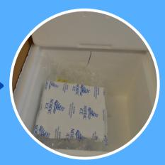
Place bubbled wrapped sample bag on bottom ice pack & add a second ice pack on top
