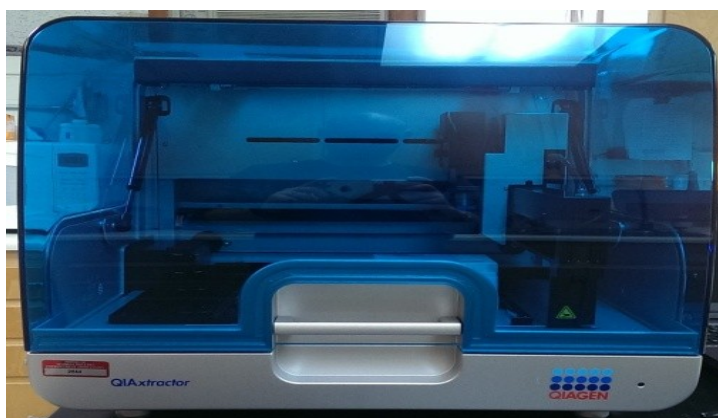
Front and Side Views of the Qiagen Extraction Automated Liquid Handling Sys-
